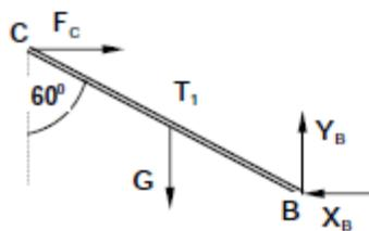
$$\begin{aligned} \sum_{i=1}^4 X_i &= 0; \quad F_C - X_B = 0; \\ \sum_{i=1}^4 Y_i &= 0; \quad Y_B - G = 0; \\ \sum_{i=1}^4 M_B^F &= 0; \quad G \frac{a}{2} \sin 60^\circ - F_C a \cos 60^\circ = 0; \end{aligned}$$
