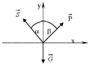
$$\begin{aligned} \sum_{i=1}^3 X_i &= 0; \quad P \sin \beta - S \sin \alpha = 0; \\ \sum_{i=1}^3 Y_i &= 0; \quad -G + P \cos \beta + S \cos \alpha = 0; \\ P &= (\sqrt{3} - 1) \cdot G \quad S = \frac{\sqrt{2}}{2} (3 - \sqrt{3}) \cdot G. \end{aligned}$$
