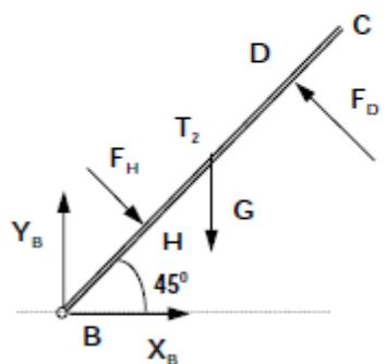
$$\overline{BH} = \frac{\sqrt{2}}{2} a, \overline{BD} = \frac{3\sqrt{2}}{2} a, \overline{BT_2} = a\sqrt{2}$$
