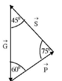
$$\begin{aligned} \frac{G}{\sin 75^\circ} &= \frac{P}{\sin 45^\circ} = \frac{S}{\sin 60^\circ} \\ \sin 75^\circ &= \sin(30^\circ + 45^\circ) = \frac{\sqrt{2}}{4} (\sqrt{3} + 1) \\ P &= (\sqrt{3} - 1) \cdot G \quad S = \frac{\sqrt{2}}{2} (3 - \sqrt{3}) \cdot G. \end{aligned}$$
