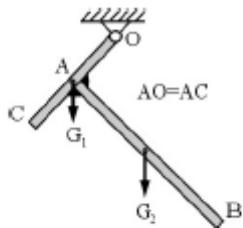
$$\begin{aligned}\sum M_{F_i}^O &= 0 \\ -G_1 \frac{l_1}{2} \cos \varphi + G_2 \left( \frac{l_2}{2} \sin \varphi - \frac{l_1}{2} \cos \varphi \right) &= 0 \\ \tan \varphi &= \frac{l_1 (G_1 + G_2)}{l_2 G_2}\end{aligned}$$
