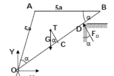
$$\begin{aligned} \sum_{i=1}^3 X_i &= 0; \quad X_0 - F_D \sin \alpha = 0; \quad \sin \alpha = \frac{4}{5} \\ \sum_{i=1}^3 Y_i &= 0; \quad Y_0 - G + F_D \cos \alpha = 0; \quad \cos \alpha = \frac{3}{5} \\ \sum_{i=1}^3 M_O^F &= 0; \quad G \cdot 3a \cdot \cos \alpha - G \cdot \frac{4}{3}a \cdot \sin \alpha - F_D \frac{11}{3}a = 0 \end{aligned}$$
