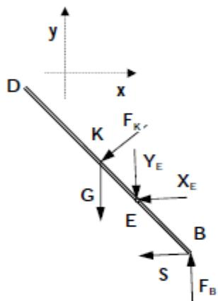
$$\begin{aligned} \sum_{i=1}^n X_i &= 0; \quad -S - X_E - F_K \frac{\sqrt{2}}{2} = 0 \\ \sum_{i=1}^n Y_i &= 0; \quad F_B - Y_E - G - F_K \frac{\sqrt{2}}{2} = 0 \\ \sum_{i=1}^n M_B &= 0; \quad -Y_E 2R \frac{\sqrt{2}}{2} - X_E 2R \frac{\sqrt{2}}{2} - G 3R \frac{\sqrt{2}}{2} - F_K 3R = 0 \end{aligned}$$
