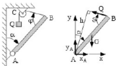
$$\begin{aligned}1) \sum F_{ix} &= 0; X_A - Q \sin(\varphi + \alpha) = 0 \\ 2) \sum F_{iy} &= 0; Y_A - G - Q \cos(\varphi + \alpha) = 0 \\ 3) \sum M_{F_i}^B &= 0; Qh - \frac{Gl \sin \alpha}{2} = 0\end{aligned}$$
