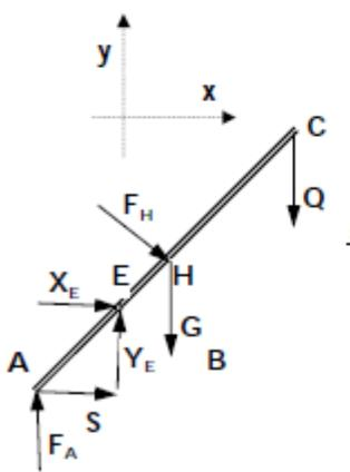
$$\begin{aligned} \sum_{i=1}^n X_i &= 0; \quad S + X_E + F_H \frac{\sqrt{2}}{2} = 0; \\ \sum_{i=1}^n Y_i &= 0; \quad F_A + Y_E - G - Q - F_H \frac{\sqrt{2}}{2} = 0 \\ \sum_{i=1}^n M_A &= 0; \quad -Y_E 2R \frac{\sqrt{2}}{2} + X_E 2R \frac{\sqrt{2}}{2} + G 3R \frac{\sqrt{2}}{2} + F_H 3R + Q 6R \frac{\sqrt{2}}{2} = 0 \end{aligned}$$
