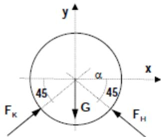
$$\begin{aligned} \sum_{i=1}^n X_i &= 0; \quad F_K \cos 45^\circ - F_H \cos 45^\circ = 0; \\ \sum_{i=1}^n Y_i &= 0; \quad -G + F_K \sin 45^\circ + F_H \sin 45^\circ = 0; \\ F_K &= \frac{\sqrt{2}}{2} G \quad F_H = \frac{\sqrt{2}}{2} G \end{aligned}$$
